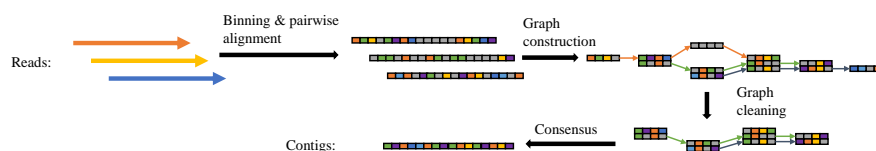
Fig. 1: The overview of the long-read assembling process in wtdbg2.
